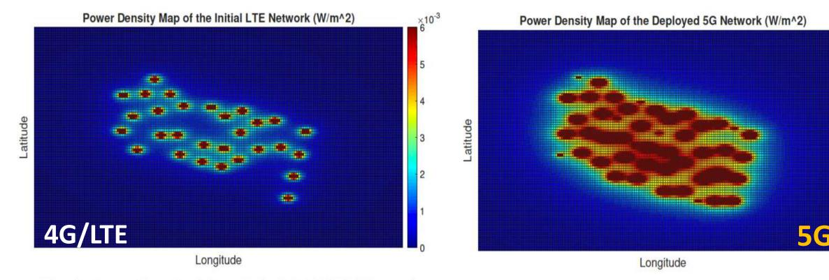
Fig. 9: Power Density Map of the Initial LTE Network
